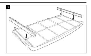
2. Position Brackets at desired position. Brackets are height and depth adjustable.
