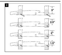
3. Attach Brackets to Sliders using 1/4" Spacers and Machine 5/8" Countersunk Screws.
